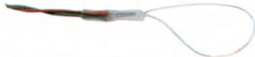
The penile strain gauge is used to measure erectile response by detecting changes in the circumference of the penis. The device is used in sexuality research.
