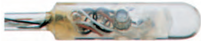
The vaginal plethysmograph is used to measure sexual response by detecting changes in the amount of blood in the vaginal walls. The device is used in sexuality research.
