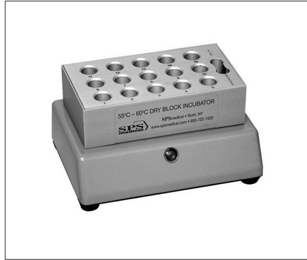
Figure 3-14 Self-contained biological incubator (note ampoule crusher to the right of the indicator wells...)
