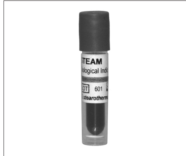
Figure 3-10 Self-contained biological indicators containing a known population of spores
