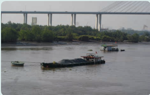
FIGURE 4-20 Two barges on the Saigon River in Vietnam, one with cargo, one without, float at different levels due to isostatic equilibrium. © Pluff Mud Photography.
