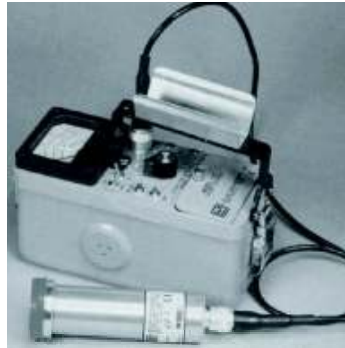
Figure 1-7 Geiger counters. (a) A pancake-type detector, useful for finding contamination. Photo courtesy of Capintec, Inc. (b) A typical Geiger–Müller tube attachment. Photo courtesy of Biodex Medical Systems, Inc.
