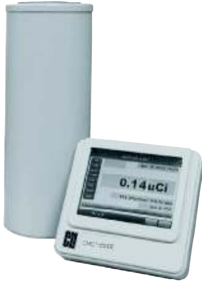
Figure 1-5 A commercial dose calibrator. One can see the shield of the ionization chamber with the dipper handle at the top, as well as the electronic readout module. Photo courtesy of Capintec, Inc.
