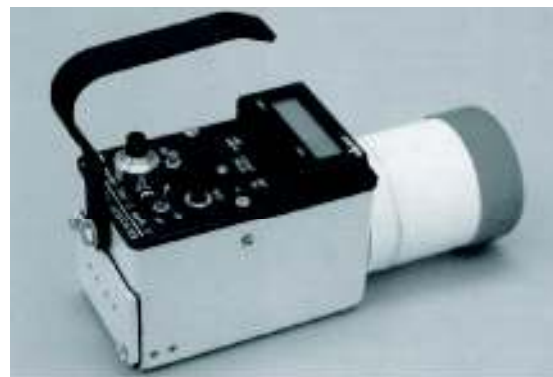
Figure 1-6 Ionization survey meter. Note the single-unit construction, which distinguishes an ionization survey meter from most Geiger counters. Photo courtesy of Biodex Medical Systems, Inc.
