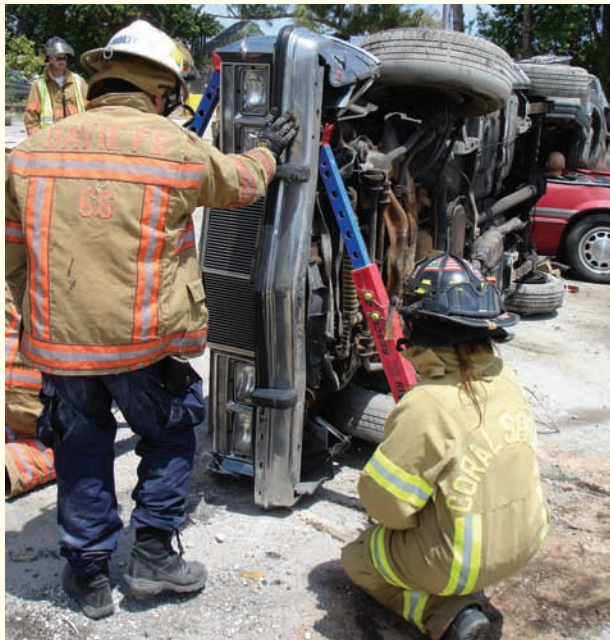
Figure 8-13 The position of the technical rescuer in charge of the operation should be at the front or rear of the vehicle; this provides full control of the operation by providing visibility to both sides of the vehicle.
