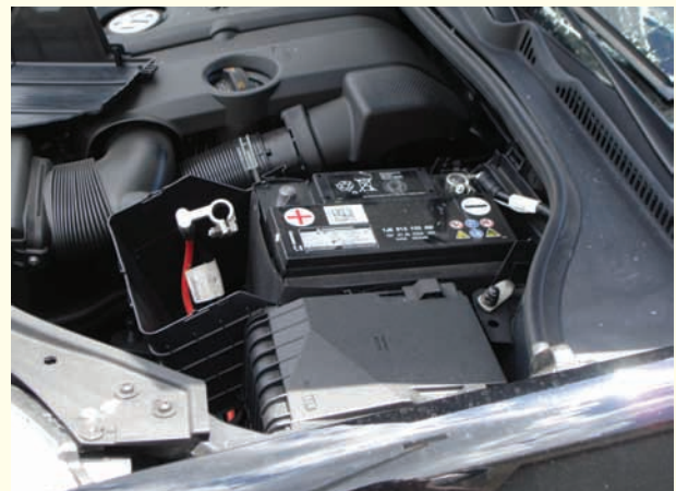
Figure 8-21 Isolating or eliminating a vehicle's electrical system may be as simple as disabling the vehicle's 12-volt DC battery, removing fuses from the fuse box, and/or removing any smart keys out of the range area.
