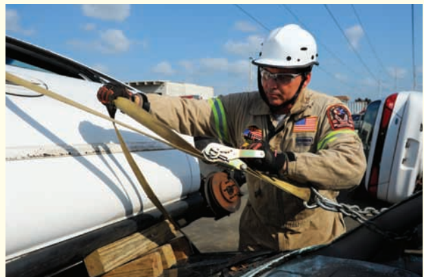
Figure 8-18 Marrying two vehicles utilizing the technique in Skill Drill 8-4 gives you access to the victim through the entire door and roof area. Even if the A-post were cut for a roof removal, the lower area of that post is strong enough to remain a solid anchor point.
