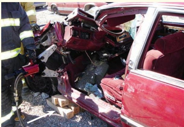
Figure 8-7 When using cribbing, whether it is a basic four-by-four or a step chock, the goal is to make the contact area from the ground to the undercarriage tight, filling up any void spaces.
