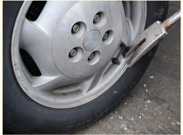
Figure 8-10 ▴ Sliding the flat section of the fork of a Halligan bar forward over the area of the rubber tire stem will cut off the end of the tire stem at the base where it protrudes from the rim.
