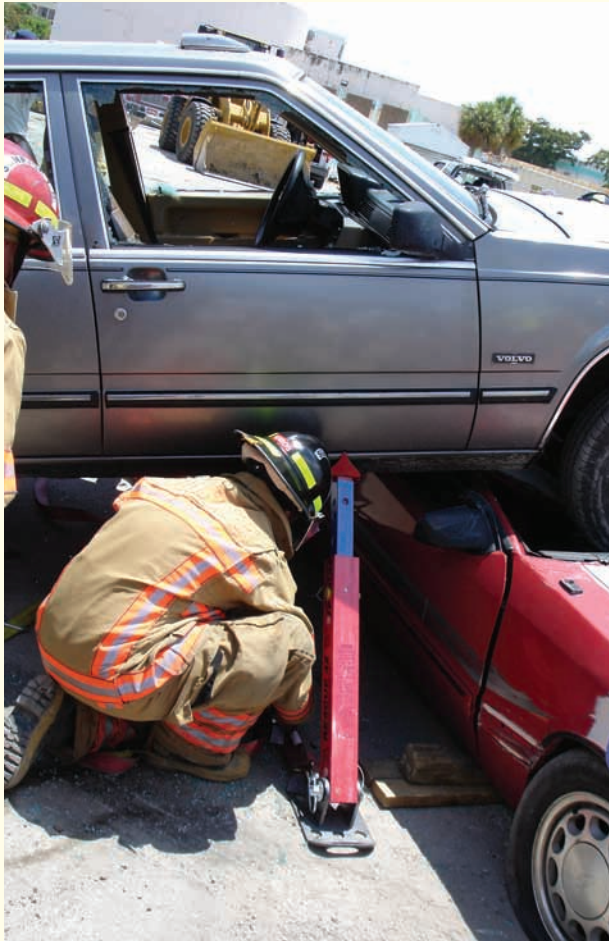
Figure 8-19 There are several additional cribbing options that can be added to the side of the vehicle on top to prevent any potential sliding as the bottom vehicle is being stabilized.
