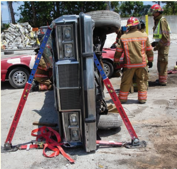
Figure 8-12 Buttress stabilization struts are structural supports that can be made of steel, aluminum, composite/Kevlar® wrap, and wood. They are used as a “buttress” to stabilize and reinforce an object, expanding a vehicle's base or footprint while also lowering its center of gravity.
