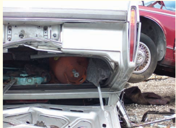
Figure 8-20 Hidden dangers such as this portable propane tank may be found in the trunk of a vehicle.
