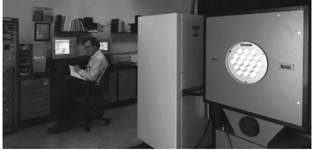
Continuous concentrator cell current versus voltage measurement test bed. The light is directed from a 1,000W xenon lamp on to a sample.
