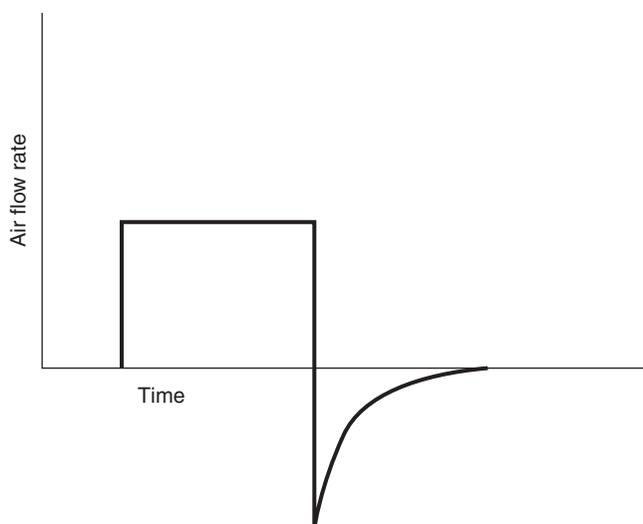
**Figure 4-2b** Volume control mode with a constant air flow rate, represented by the square waveform seen here. Constant air flow continues until the set  $V_t$  is delivered.
