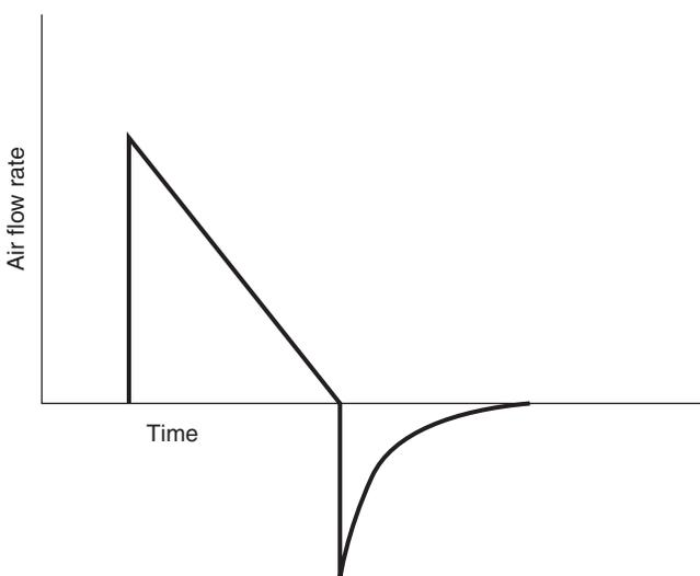
**Figure 4–2a** Pressure control with a decelerating air flow rate. A constant pressure is maintained in the ventilator circuit and a resulting  $V_t$  is delivered.
