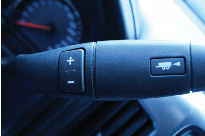
FIGURE 11-23 Manual transmission control buttons installed on the shift lever on a late-model pickup truck.
