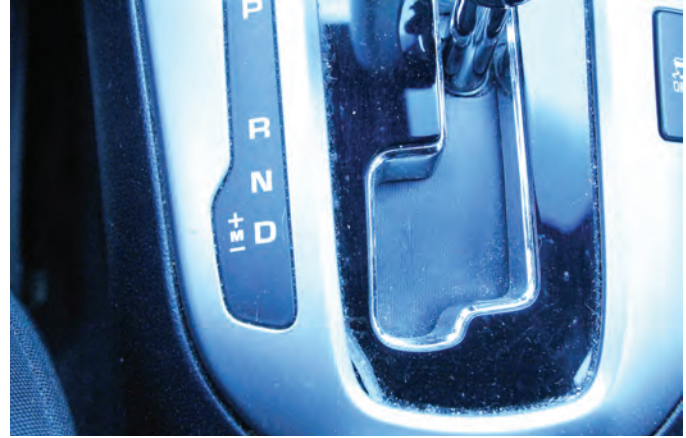
FIGURE 11-24 A floor-mounted gear shift that allows manual operation.
