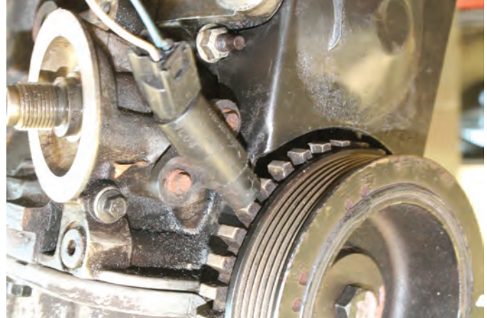
FIGURE 11-18 A crankshaft position (CKP) sensor installed on the front of a crankshaft.
