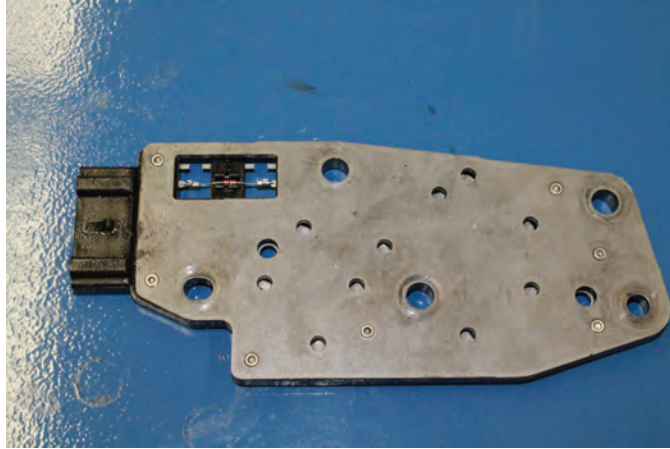
FIGURE 11-8 A General Motors TFT sensor and pressure switch assembly.
