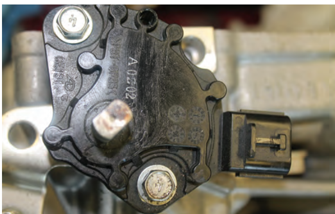
FIGURE 11-21 A manual lever position (MLP) switch mounted on the outside of the transmission. Note the manual lever linkage passing through the middle of the switch.
