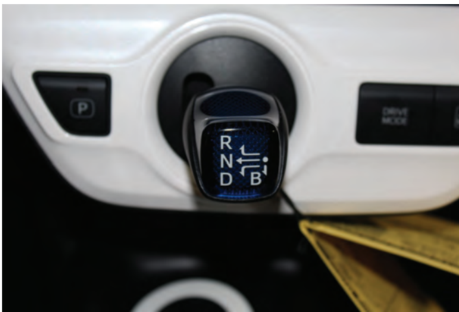
FIGURE 11-39 Regeneration Mode on this Prius Hybrid vehicle is activated by the shift selector.
