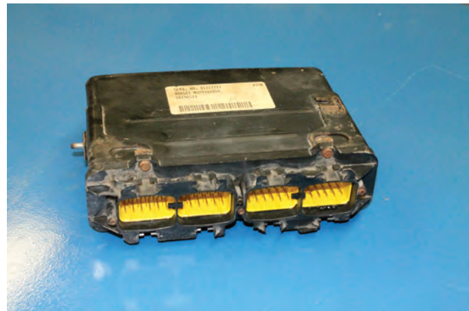
FIGURE 11-2 A typical vehicle PCM that has been removed from a vehicle.
