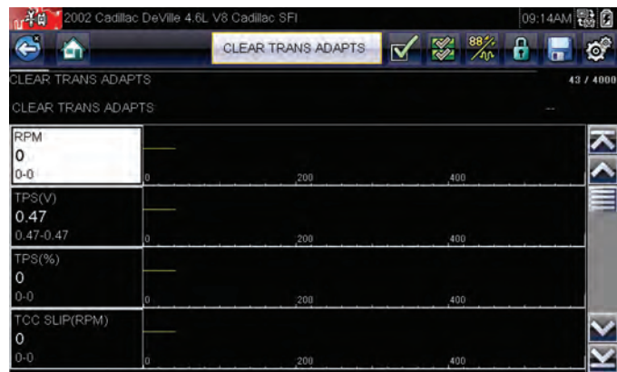
FIGURE 11-42 Transmission adaptive pressure being reset after a transmission repair.
