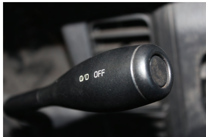
FIGURE 11-22 An overdrive switch used by the driver to manually select or deselect overdrive.
