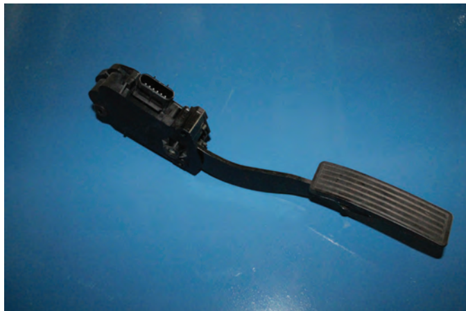
FIGURE 11-14 Accelerator pedal position sensor.
