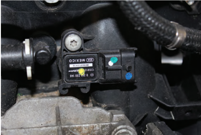
FIGURE 11-16 A common MAP sensor installed on an intake manifold.
