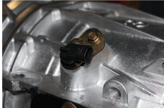
FIGURE 11-6 An input shaft speed sensor on an Allison 1000 transmission. This sensor will measure the speed of the Power Take Off (PTO) gear that is part of the input shaft of this transmission. You can see the teeth of the PTO gear through the hole in the case.
