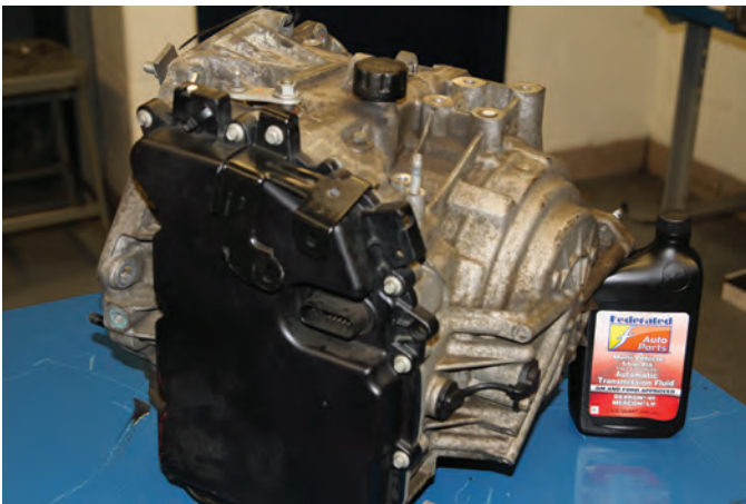
FIGURE 11-1 A typical electronically controlled transmission removed from a vehicle.
