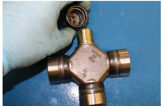
FIGURE 8-5 Needle bearings used in Cardon U-joint.
