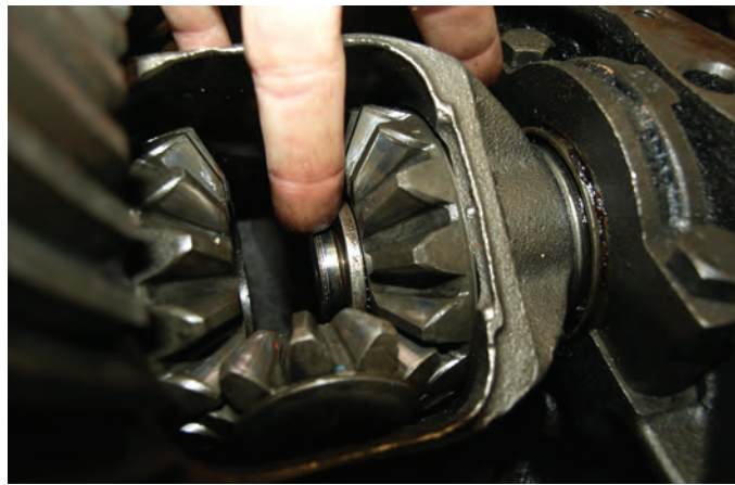
FIGURE 8-4 C-lock differential axle retention.
