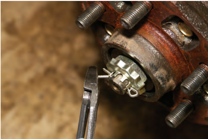
FIGURE 8-17 Typical cotter pin-style wheel bearing locking mechanism.
