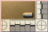
Figure 4.10 Proper use of ABFO scale as to plane and camera angle (props used to raise scale). Culotta, A.W. (2013) Basic Crime Scene Photography, 2nd Ed.
