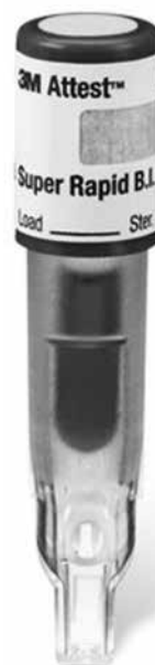
Figure 3-20 Rapid Readout Biological Monitor. Courtesy of 3M, St. Paul, MN. The image is reproduced herein with permission. © 3M, 2013. All rights reserved.
