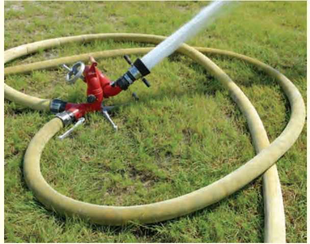
FIGURE 22-7 A portable monitor is placed on the ground and supplied with water from one or more hose lines.
