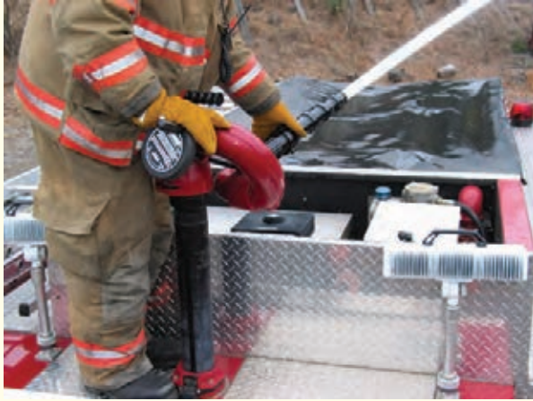
FIGURE 22-6 A deck gun is permanently mounted on a vehicle and equipped with a piping system that delivers water to the device.
