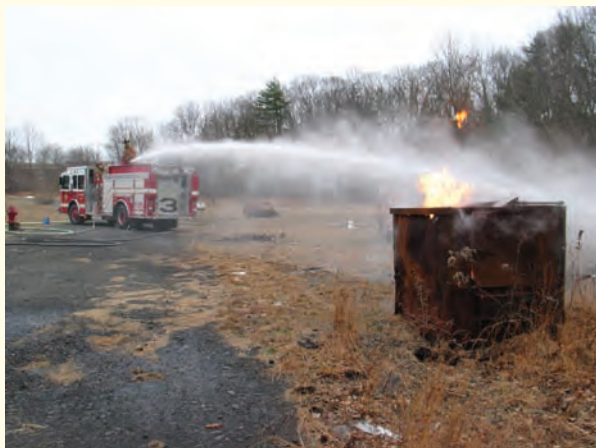
FIGURE 22-12 Some fire departments use a deck gun on top to extinguish large trash container fires.
