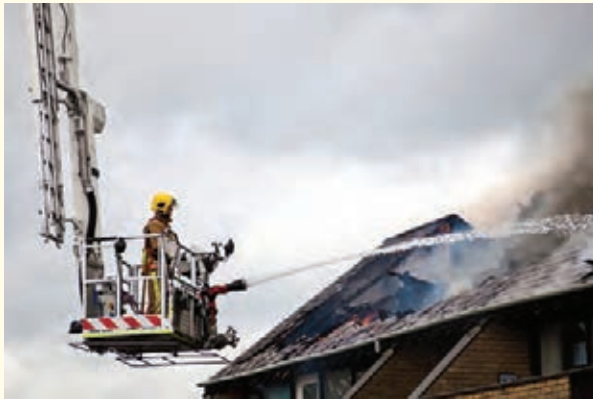
FIGURE 22-8 Elevated master stream devices can be mounted on aerial apparatus.
