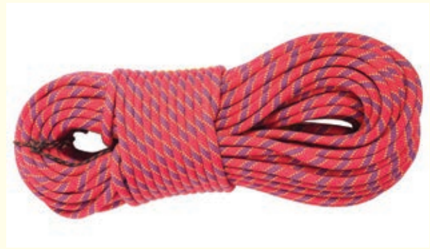
FIGURE 10-20 Ropes may be coiled for storage.
