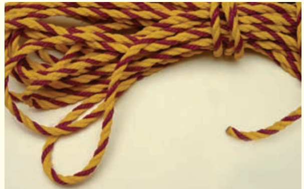
FIGURE 10-7 Polypropylene rope is often used in water rescues.
