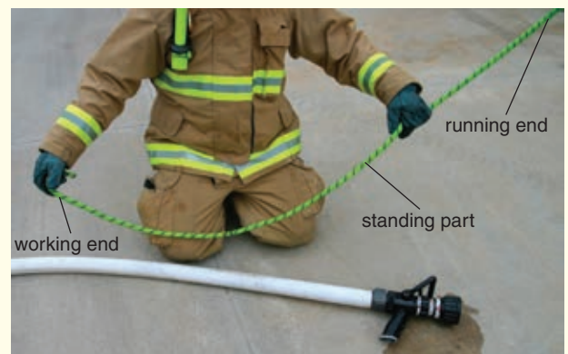
FIGURE 10-22 The sections of a rope used in tying knots.
