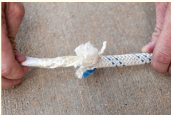
FIGURE 10-9 The parts of a kernmantle rope.
