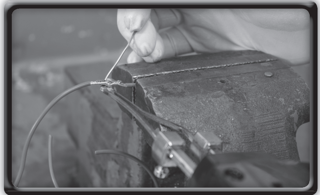
_____ D. Apply the hot solder iron tip to heat the joint, then apply solder to the joint (not the iron). If the solder does not melt within a few seconds, remove it and allow the joint to heat further before reapplying.
