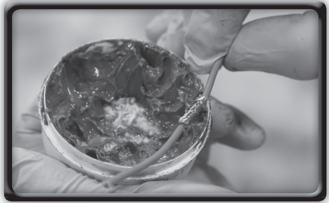
_____ B. Apply flux to the wires or metal to be soldered. This may not be necessary if you are using cored solder.
