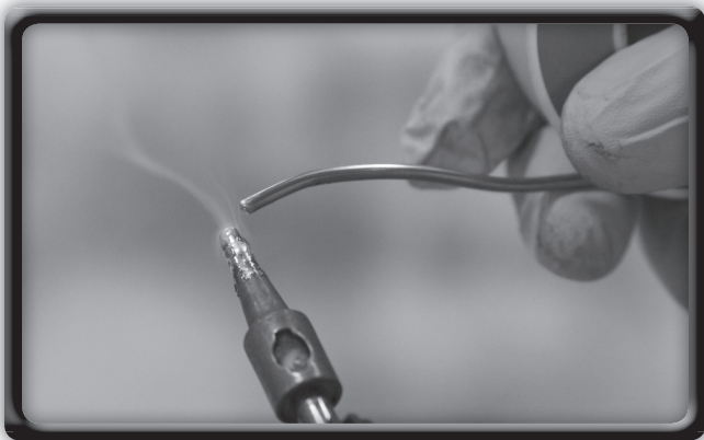
_____ E. Prepare the soldering iron by ensuring the correctly sized tip is fitted and is clean. Tin the soldering iron tip by melting some solder to it and wiping any excess from the tip.
