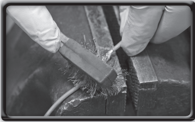
_____ A. Clean any excess flux from the joint.
