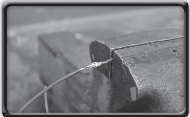
_____ F. Once the solder has been applied, ensure the joint does not move until the solder has cooled sufficiently to set. Once cooled, inspect the joint; it should be shiny and firm.
