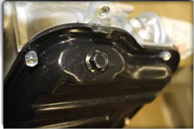
FIGURE 12-7 A drain plug allows oil to be drained during oil changes.
