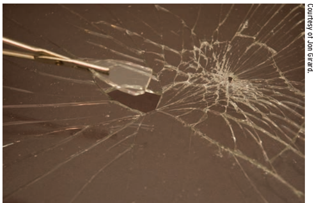
FIGURE 5-2 Matching broken pieces of glass. Finding a perfect match is tantamount to individualizing the glass to a single source with complete certainty.
