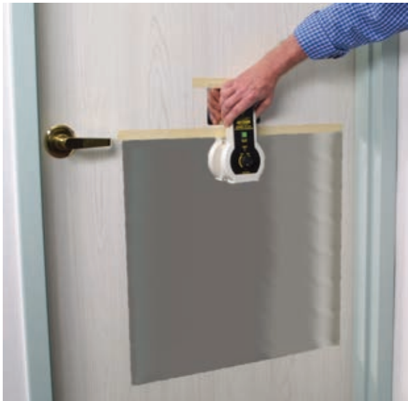
FIGURE 2-7 The electrostatic plate will lift dust from horizontal and vertical surfaces, thereby recording the impression.
