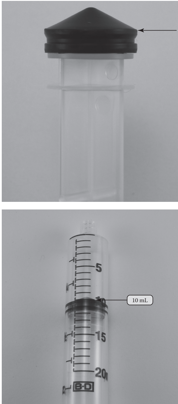
Figure 2-8 Final Edge of Piston Plunger Used for Measuring
