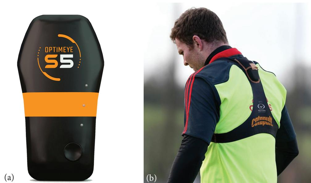
**Figure 1.6** (a) A GPS receiver used to track player motion. (b) The receiver is housed in a vest worn by the player.
