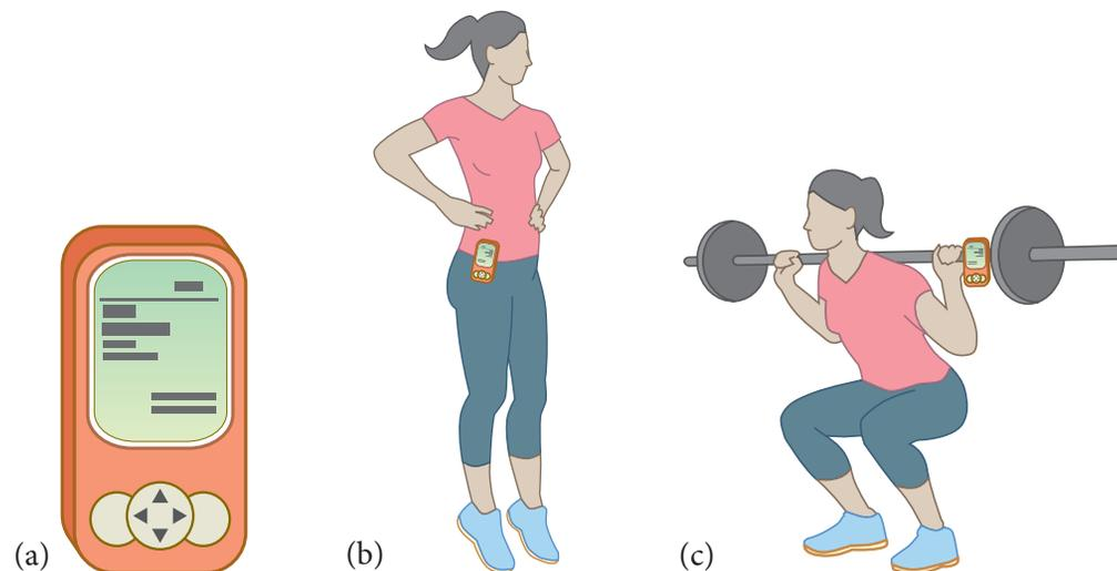
**Figure 1.8** (a) An accelerometer used to assess movements. (b) An accelerometer attached to an athlete during a vertical jump test. (c) An accelerometer attached to the barbell during a resistance exercise.
