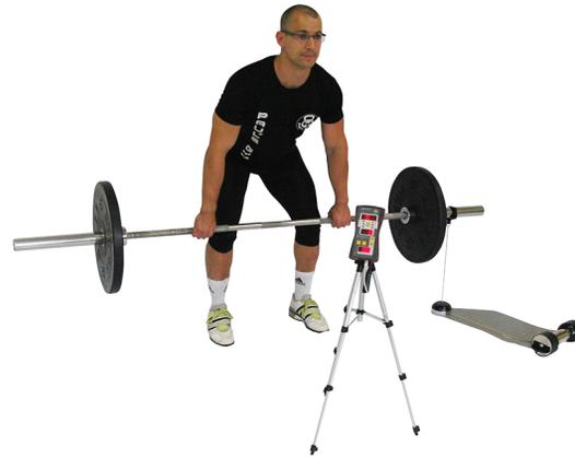
**Figure 1.7** A linear position transducer attached to a barbell via a cable is used to record the velocity of the barbell during a snatch movement.
