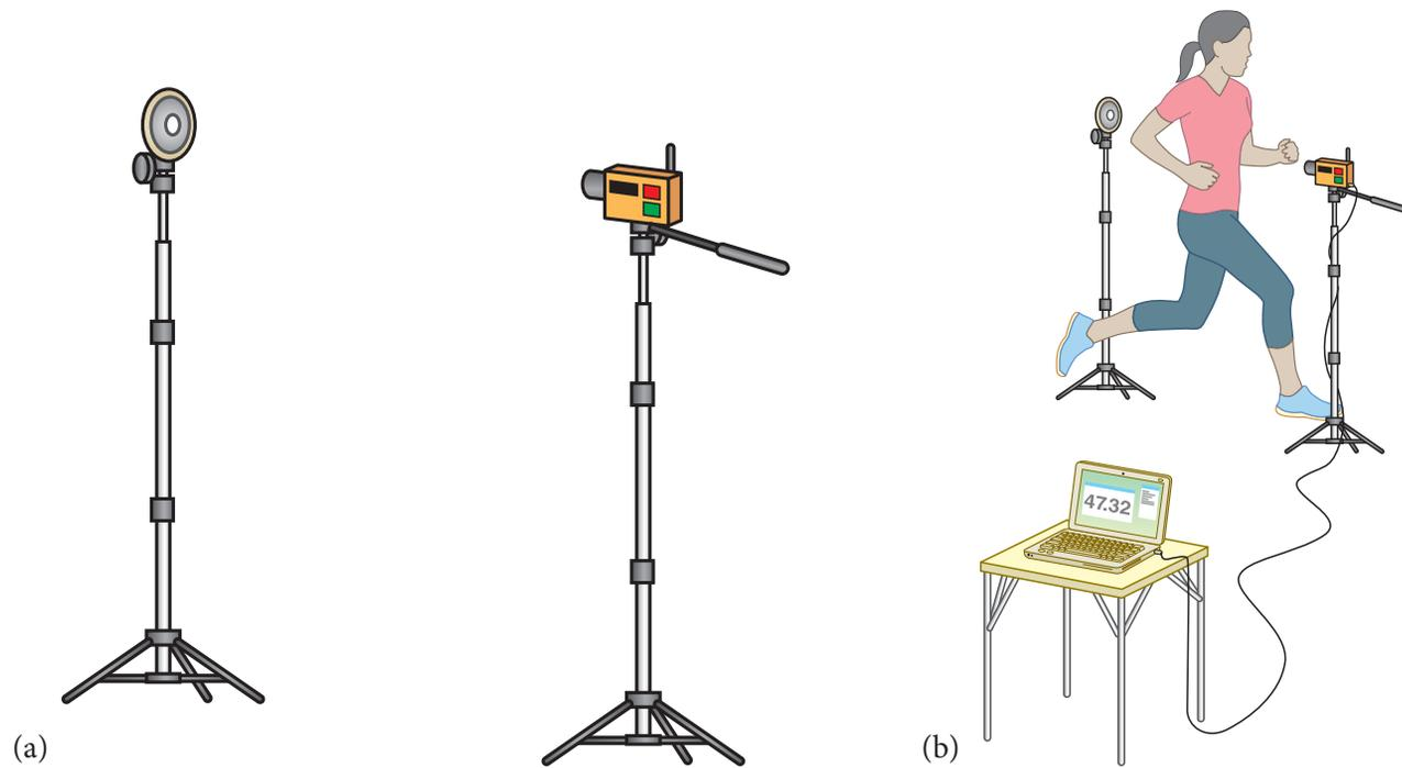
**Figure 1.4** Timing gates used to record running speed. (a) An emitter–reflector pair. An infrared beam from the emitter (foreground) is reflected back from the reflector placed directly opposite. The interruption of the beams associated with timing gates set at known distances along the path of motion allows the determination of speed. (b) The use of photocells to record the sprinting speed of an athlete.
