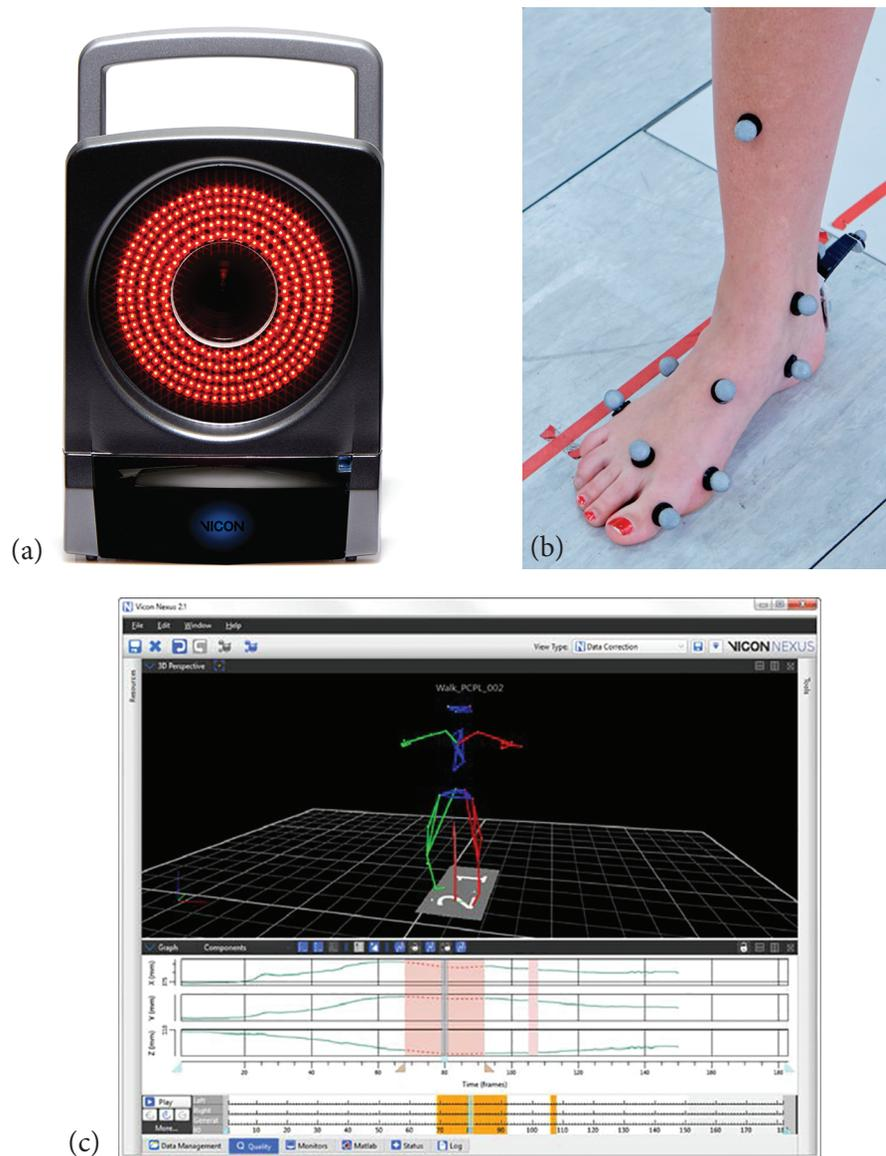
**Figure 1.10** (a) An opto-reflective camera with an LED array. (b) Reflective markers placed on anatomical landmarks to allow the body segments to be located within three-dimensional space. (c) The digital output obtained from a three-dimensional opto-reflective motion analysis system.
