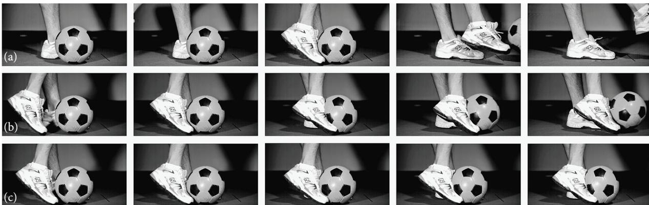
**Figure 1.9** The effects of different sampling frequencies in the motion analysis of a soccer kick using a two-dimensional video-based motion analysis system. (a) At a sampling frequency of 50 Hz, foot–ball contact can be observed in only one frame. (b) At a sampling frequency of 250 Hz, foot–ball contact is observed in four frames. (c) At a sampling frequency of 1000 Hz, foot–ball contact is observed in many frames.
