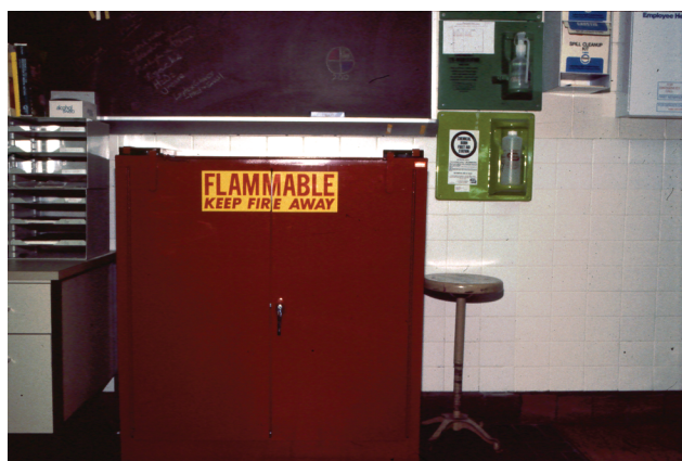
FIGURE 2-5 Chemical storage cabinet
