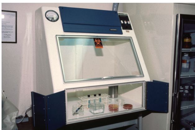
FIGURE 2-3 Class II biological safety cabinet
