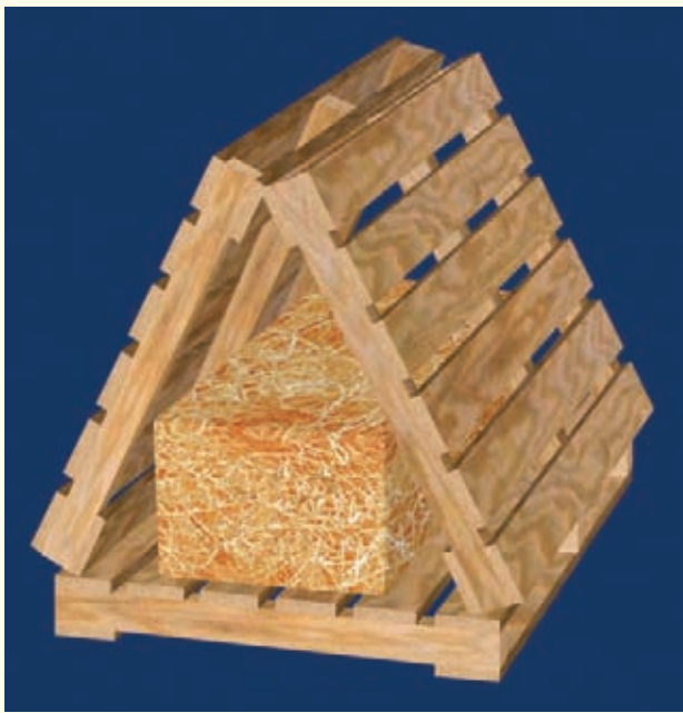
Figure 6-16 One method for configuring the burn set is to lean two pallets against each other, forming a triangle, and place hay or excelsior in the middle.
