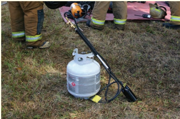
Figure 6-17 A propane torch can be used for interior ignition.
