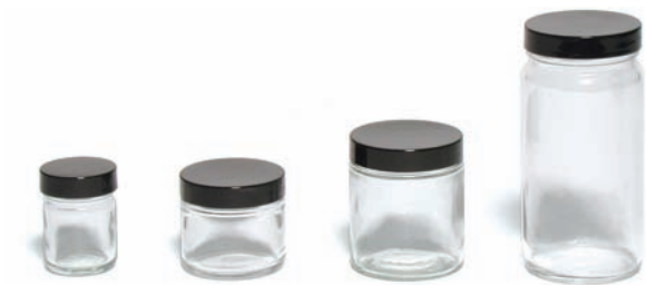
FIGURE 1-11 Wet or liquid samples may be placed in airtight jars. After the top is screwed on, the jar should be sealed with tape to prevent contamination.
