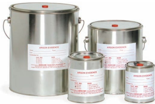
FIGURE 1-12 Once the lid is in place, an airtight seal prevents evaporation of liquid evidence. The rubber septum in the lid later may be punctured with a syringe to take a sample for analytical purposes.
