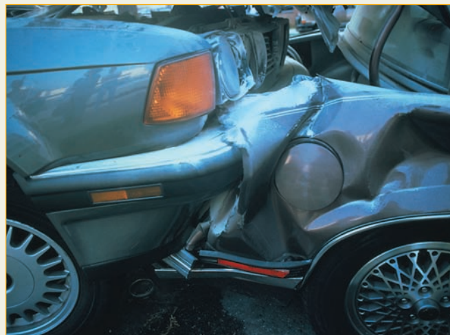
Figure 17-5 The kinetic energy of a speeding car is converted into the work of stopping the car, usually by crushing the car's exterior.
