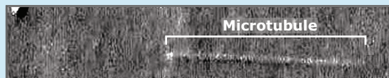
FIGURE 11.B1 A microtubule viewed by differential interference contrast (DIC) microscopy and computer image enhancement. The image is grainy, but the position and length of the microtubule are clear. This form of microscopy can be used to measure how long microtubules are, watch them move, or watch particles move along them. Photo courtesy of Lynne Cassimeris, Lehigh University.
