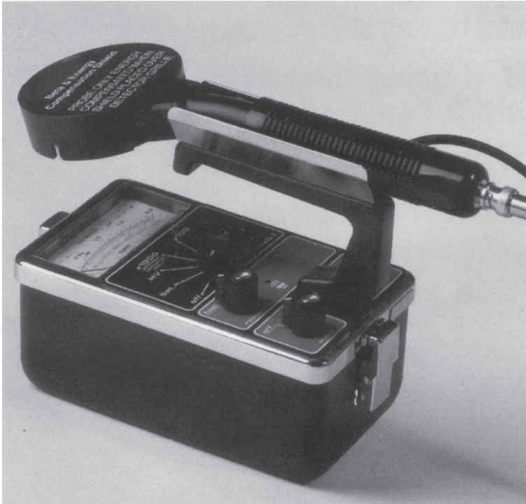
Figure 1-7 Geiger counters. Figure 1-7a shows a pancake-type detector, useful for finding contamination. Photo courtesy of Capintec, Inc. Figure 1-7b shows a typical Geiger-Müller tube attachment. Photo courtesy of Biodex Medical Systems, Inc.
