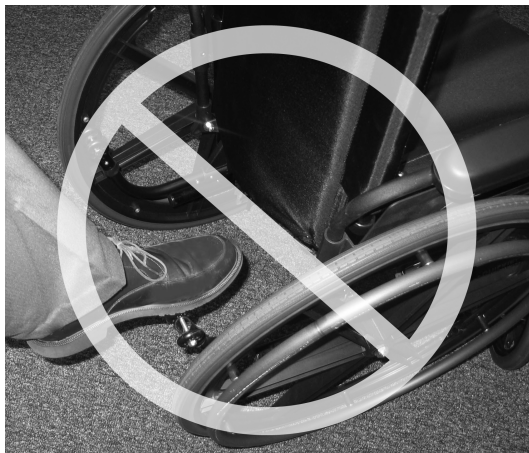
FIGURE 11-2 Avoid stepping on rear anti-tippers because they easily break.
