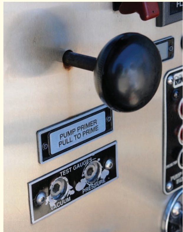
Figure 6-22 A priming pump is used to draw air out the centrifugal pump.
