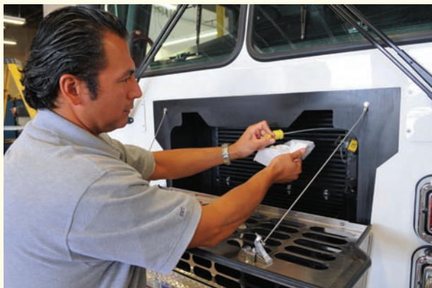
Figure 6-10 Access doors on newer fire apparatus allow you to inspect the fluids in the engine compartment without having to lift the cab.
