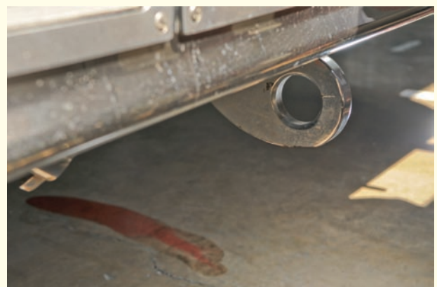
Figure 6-20 Water or other liquids dripping from underneath the fire apparatus should be inspected to determine whether the leak is serious.
