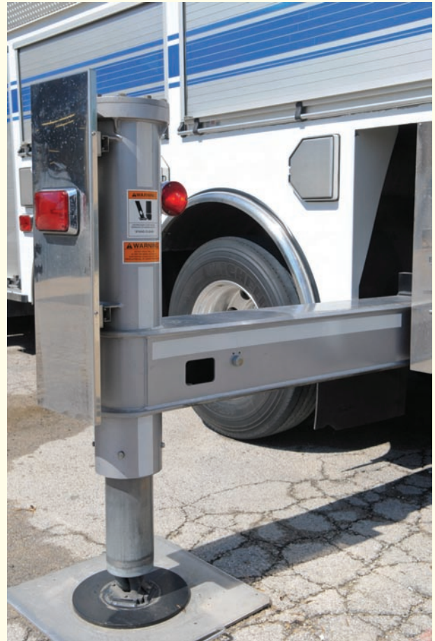
Figure 6-23 Clean stabilizers are easier to inspect for defects.
