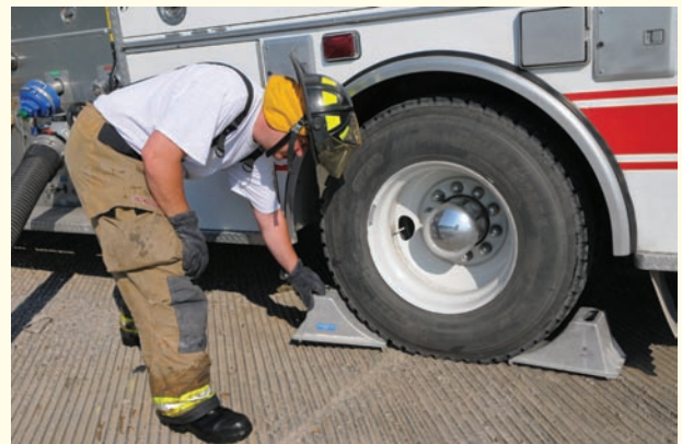
Figure 6-16 Chock the wheels of the fire apparatus when conducting a dual air brake system warning and buzzer test.
