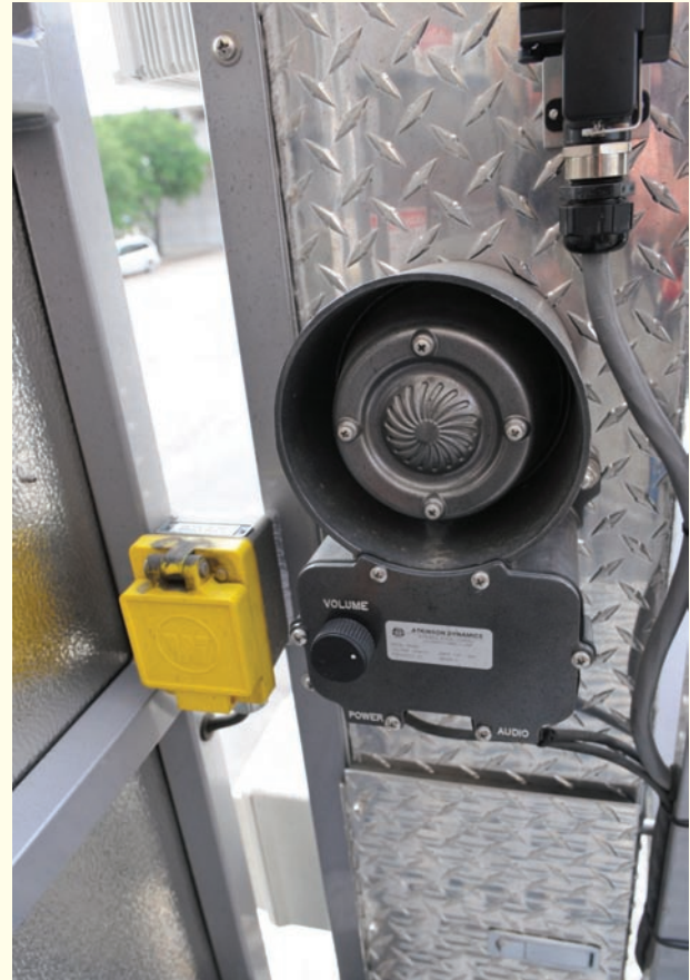
Figure 6-25 A communication system allows the driver/operator at the turntable to remain in contact with the crew members who are working at the tip of the aerial device.
