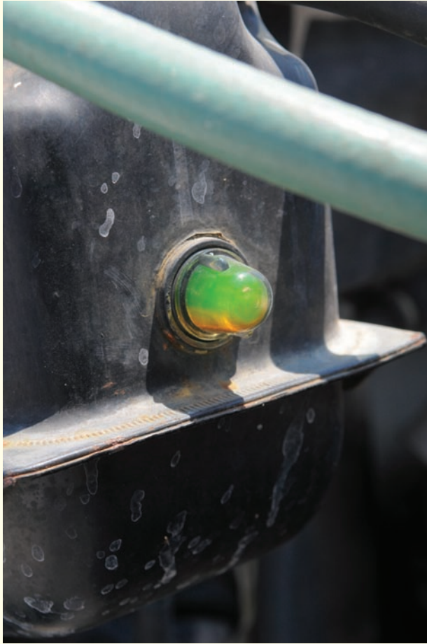
Figure 6-12 ▲ A sight glass can be very useful to check the coolant levels.
