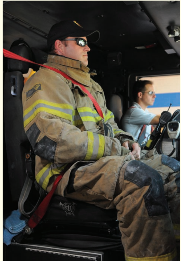
Figure 6-14 NFPA 1901 requires that seat belts be red or orange so that fire fighters can tell them apart from the waist belts on SCBA units.
