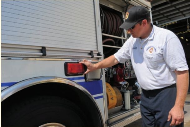
Figure 6-15 You will have to walk around the fire apparatus and visually inspect the operation of the lights on the fire apparatus.
